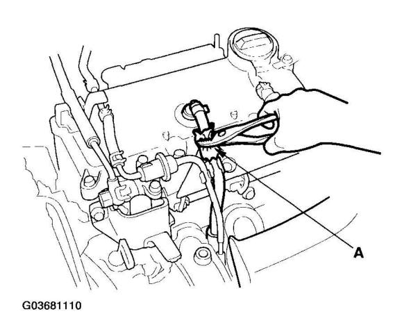
Fig. 3: Pinching Hose Between PCV Valve And Intake Manifold (2000-
