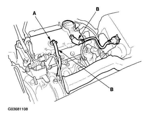
Fig. 1: Checking PCV Valve, Hoses And Connections (2000-2004 Models) Courtesy of AMERICAN HONDA MOTOR CO., INC.
