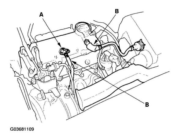
Fig. 2: Checking PCV Valve, Hoses And Connections (2005-2006 Models) Courtesy of AMERICAN HONDA MOTOR CO., INC.
