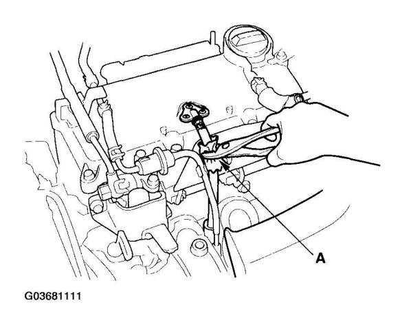
Fig. 4: Pinching Hose Between PCV Valve And Intake Manifold (2005-2006 Models)
