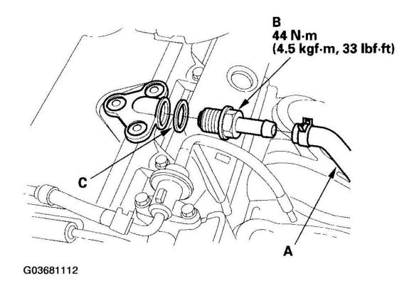
Fig. 5: Removing PCV Valve And Torque Specifications Courtesy of AMERICAN HONDA MOTOR CO., INC.
