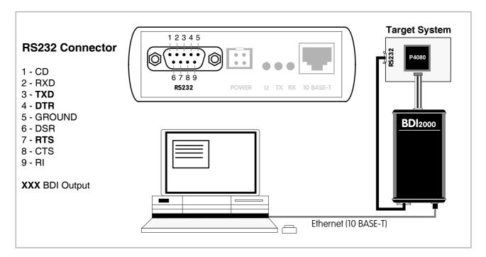
The configuration parameter "SIO" is used to enable this serial I/O routing. The used framing parameters are 8 data, 1 stop and not parity. The BDI asserts RTS and DTR when a TCP connection is established.
