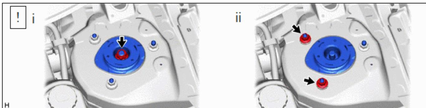
(1) Fully tighten the front support to front shock absorber nut.
