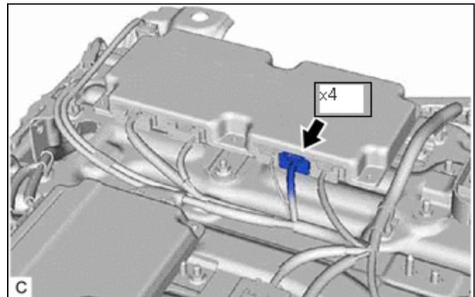
(c) Disconnect the air conditioning pressure sensor connector.
