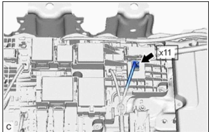
(c) Reconnect the battery ECU assembly connector.
