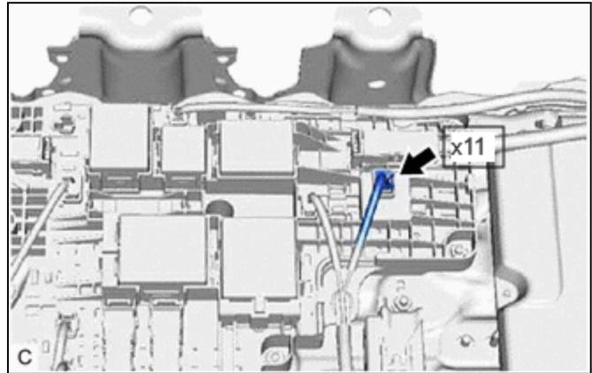
(c) Reconnect the battery ECU assembly connector.
