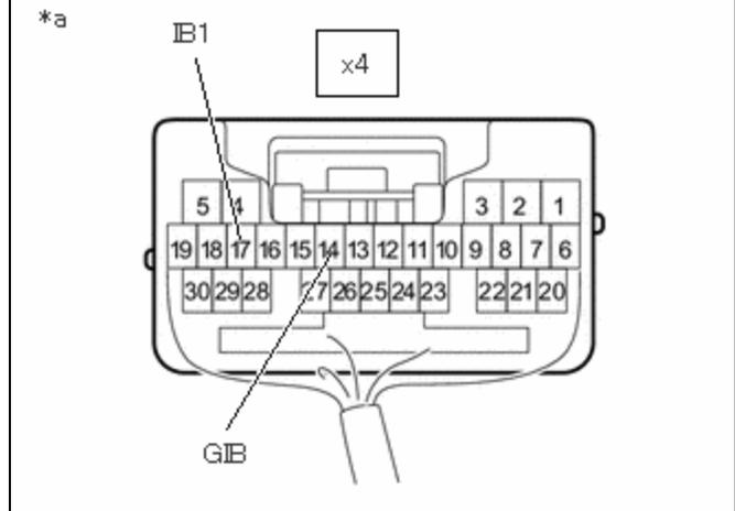
\*a Component with harness connected (Battery ECU Assembly)
