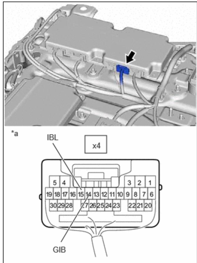
\*a Component with harness connected (Battery ECU Assembly)
