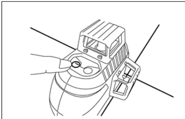
2. Align the laser beam ground marking point (cross portion) with point B.
