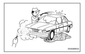
In the symptom simulation test, the problem symptoms as well as the problem area or parts must be confirmed. First, narrow down the possible problem circuits according to the symptoms. Then, connect the tester and carry out the symptom simulation test, judging whether the circuit being tested is defective or normal. Also, confirm the problem symptoms at the same time. Refer to the problem symptoms table for each system to narrow down the possible causes.
