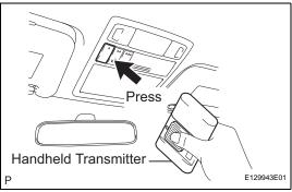
(4) When the indicator light begins to flash more rapidly, release both switches. This indicates that the garage door opener system has been successfully programmed. If the garage door opener system fails to program, review all hints before trying the programming process again.
