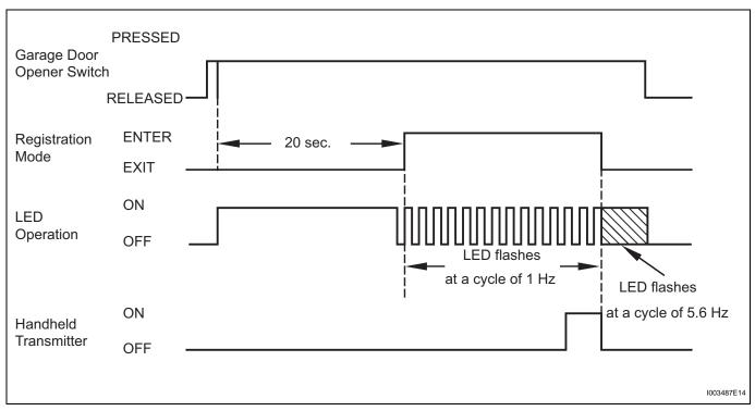
(b) Erasure of transmitter codes in the garage door opener system. (clear mode) HINT:
