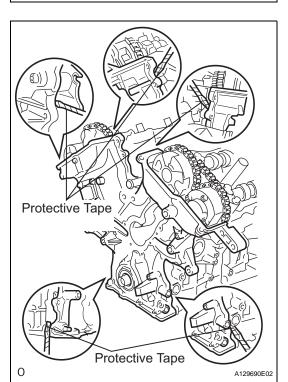
(b) Remove the timing chain cover by prying between the timing chain cover and cylinder head or cylinder block with a screwdriver.
