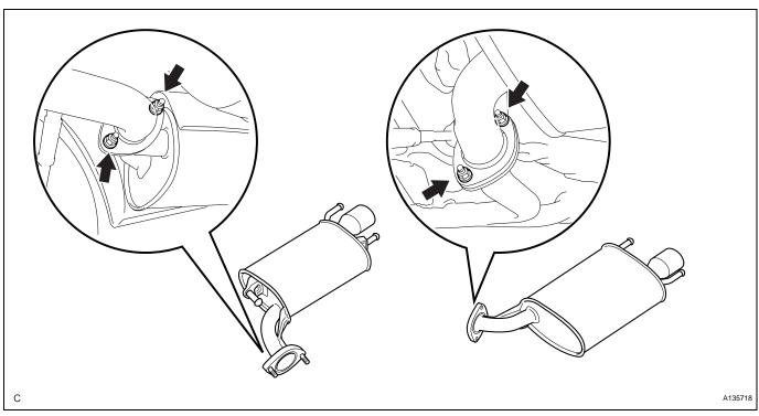
(b) Remove the 2 gaskets from the exhaust center pipe assembly.
