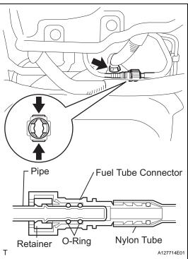
(a) Connect the main tube connector to the pipe. Push the 2 parts together firmly until a "click" sound is heard.
