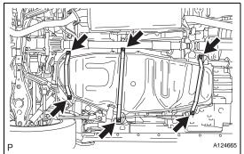
(f) Install the 3 fuel tank bands with the 6 bolts.
