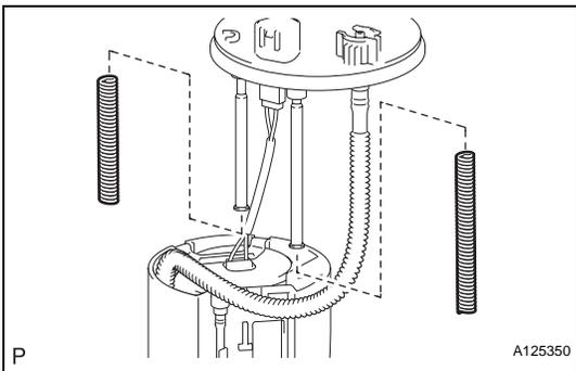
(c) Remove the 2 springs from the 2 shaft.
