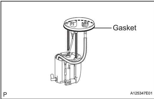
(b) Remove the gasket from the fuel pump.
