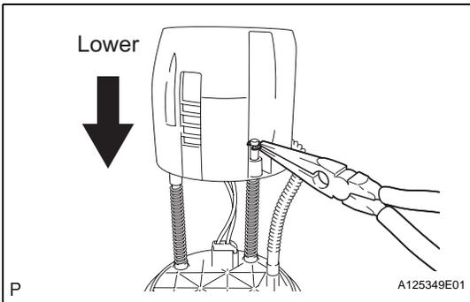
(b) Using needle nose pliers, remove the E-ring.
