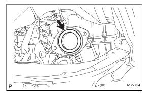
(c) Remove the gasket from the front exhaust pipe.
