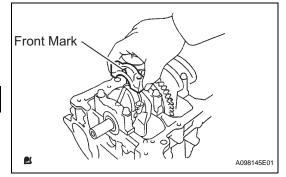
(d) Check that the front mark of the connecting rod cap is facing in the correct direction.
