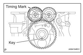
(g) Confirm that the timing marks of the balance shafts are aligned when the key groove is placed at the 6 o'clock position, as shown in the illustration.
