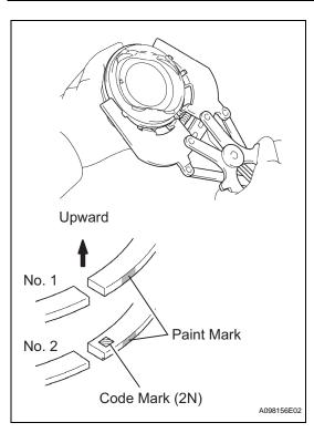
(b) Using a piston ring expander, install the 2 compression rings with the paint mark as shown in the illustration.
