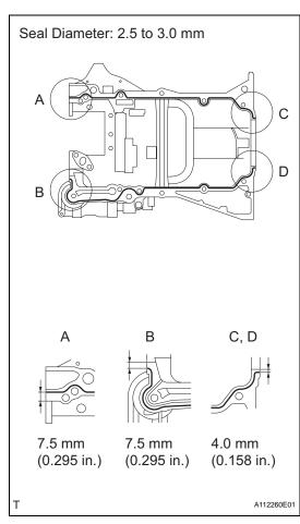
(d) Apply a continuous bead of seal packing (Diameter 2.5 to 3.0 mm (0.098 to 0.118 in.)) as shown in the illustration.
