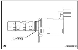
(b) Install the camshaft timing oil control valve with the bolt.
