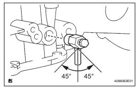
(b) After tightening the drain cock to the specified torque, turn the drain cock clockwise as shown in the illustration.
