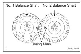
(b) Confirm that the timing marks on the No. 1 and No. 2 driven gears are aligned.
