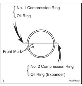
(c) Position the piston rings so that the ring ends are as shown in the illustration.
