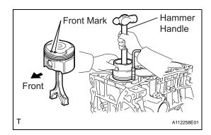
(c) Using a hammer handle and piston ring compressor, press a piston and connecting rod into each cylinder with the front mark of the piston facing forward.
