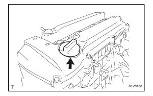
(b) Install the oil filler cap.
