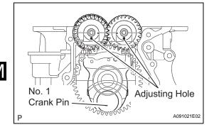
(c) With the No. 1 crank pin of the crankshaft placed at the 6 o'clock position, install the No. 1 and No. 2 balance shafts and align the adjusting holes as shown in the illustration.
