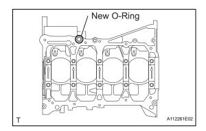
(b) Place a new O-ring on the cylinder block as shown in the illustration.
