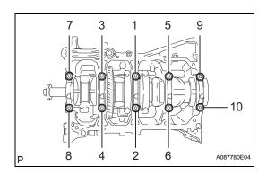
(d) Using several steps, uniformly install and tighten the 10 bearing cap bolts in the sequence shown in the illustration.
