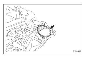
Remove the gasket from the intake manifold.
