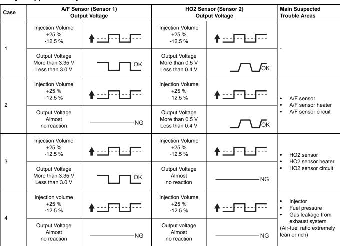
Following the A/F CONTROL procedure enables technicians to check and graph the voltage outputs of both the A/F and HO2 sensors.
