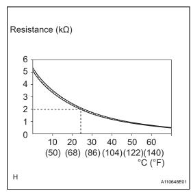
The battery temperature sensor installed on the battery current sensor detects battery temperature.
