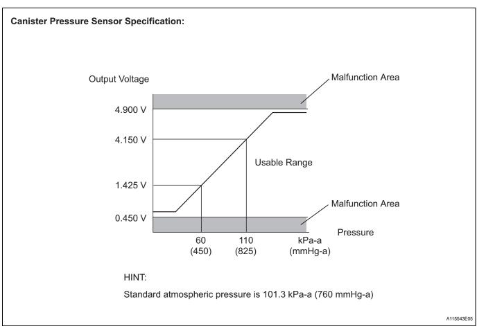
1. DTC P0450: Canister pressure sensor abnormal fluctuation
