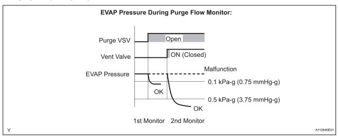
The purge flow monitor consists of the two step monitors. The 1st monitor is conducted every time and the 2nd monitor is activated if necessary.
