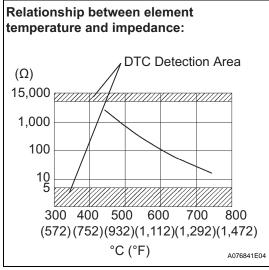
During normal air-fuel ratio feedback control, there are small variations in the exhaust gas oxygen concentration. In order to continuously monitor the slight variations in the HO2 sensor signal while the engine is running, the impedance\* of the sensor is measured by the ECM. The ECM determines that there is a malfunction in the sensor when the measured impedance deviates from the standard range.
