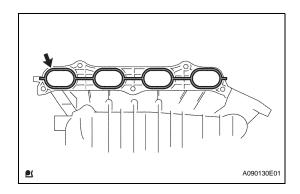
(f) Remove the gasket from the intake manifold.
