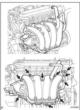
(b) Install the intake manifold with the 5 bolts and 2 nuts.
