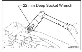
(b) Using a 22 mm deep socket wrench, remove the ventilation valve.
