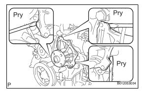
(d) Using a screwdriver, pry between the water pump and cylinder block, and then remove the water pump.
