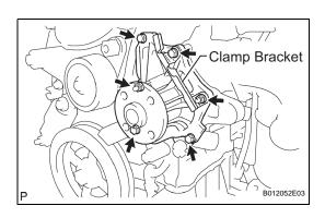
(c) Remove the 4 bolts, 2 nuts and clamp bracket.
