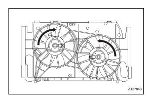
(c) Check that the cooling fan rotates.
