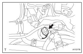
If it does not, check the fuses, cooling fan relays, ECM and cooling fan, and then check for an open circuit between the cooling fan relay and engine coolant temperature sensor.
