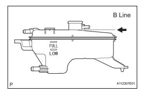
(d) Continue adding TOYOTA SLLC until it is filled to the B line at the base of the reservoir's filler neck. HINT:
