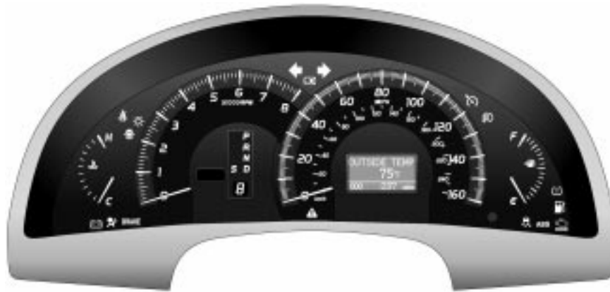
Optitron Display Type Combination Meter (XLE Grade Models with 2GR-FE Engine for U.S.A.)
