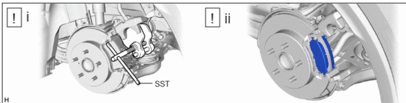
(1) Using SST, push in the rear disc brake piston.
