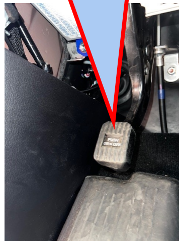
Foot Pedal for Parking Brake
