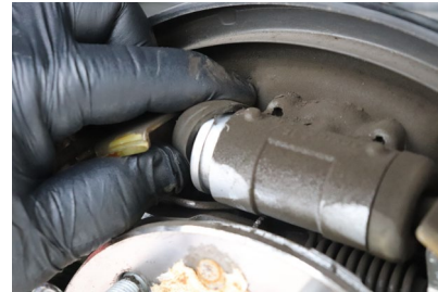
Inspecting for wheel cylinder leakage
