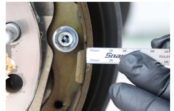
Measuring brake lining with steel ruler
