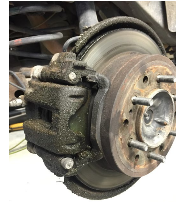
Example of leaking caliper
