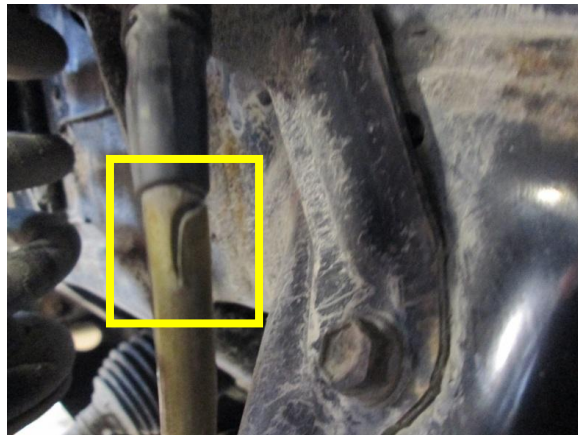
Cracked / split brake hose
