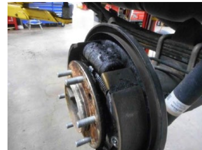
Lining contaminated with brake fluid
