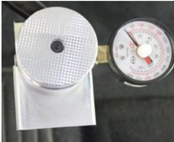
Brake Pedal Force Gauge SST P/N 09709-00002
