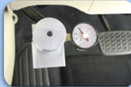
Brake Pedal Force Gauge SST P/N 09709-00002
