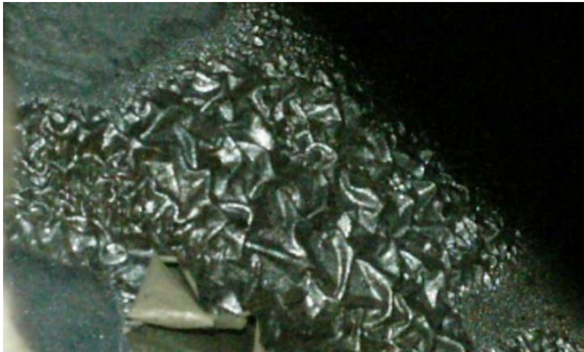
Paint Damage from Brake Fluid
