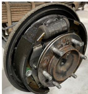
Lining contaminated with axle lubricant
