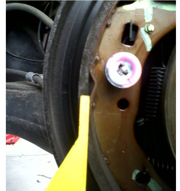
Measuring brake lining with thickness gauge
