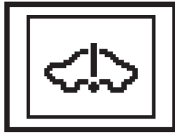
HV System Warning
