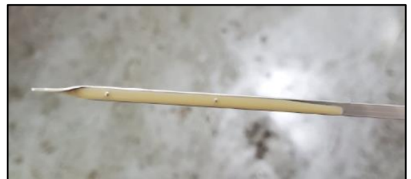
Figure 2. Engine Oil (Milky/Discolored)
