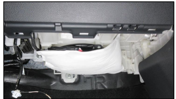
Figure 2. Incorrect Installation of Heater Cover
