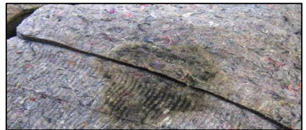
Figure 4. Examples of Organic Matter Growth due to Water Intrusion Found During Vehicle Inspection
