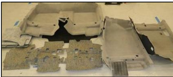
Figure 4. Examples of Organic Matter Growth due to Water Intrusion Found During Vehicle Inspection
