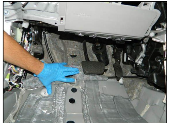
Figure 5. Driver Side Dash Panel Insulator Assembly Inspection
