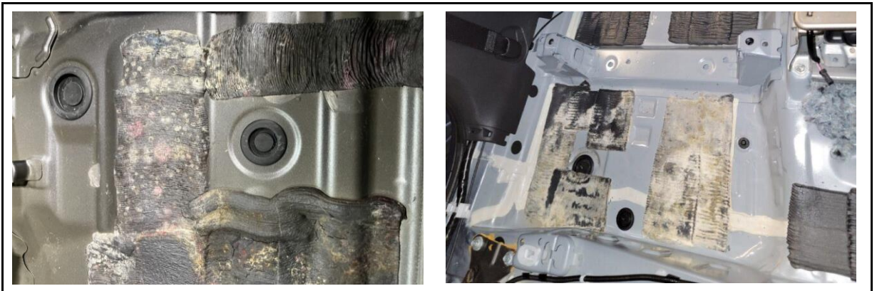
Figure 4. Examples of Organic Matter Growth due to Water Intrusion Found During Vehicle Inspection
