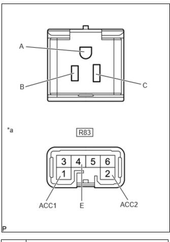
\*a Component without harness connected (Rear No. 1 Power Outlet Socket Assembly)
