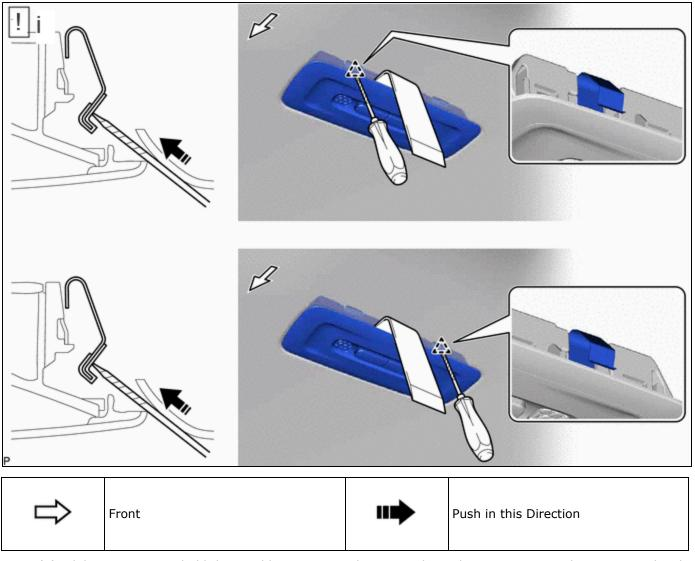
(1) While continuing to hold the moulding remover, disengage the 2 clips using a screwdriver wrapped with protective tape.
