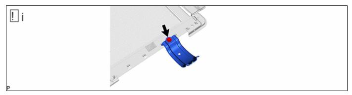
(1) Temporarily install the front sliding roof housing mounting bracket LH to the sunshade housing assembly with the bolt.
