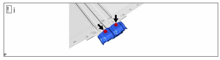
(1) Temporarily install the center sliding roof housing mounting bracket LH to the sunshade housing assembly with the 2 bolts.
