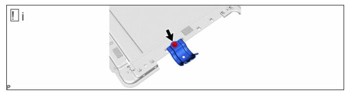
(1) Temporarily install the rear sliding roof housing mounting bracket LH to the sunshade housing assembly with the bolt.
