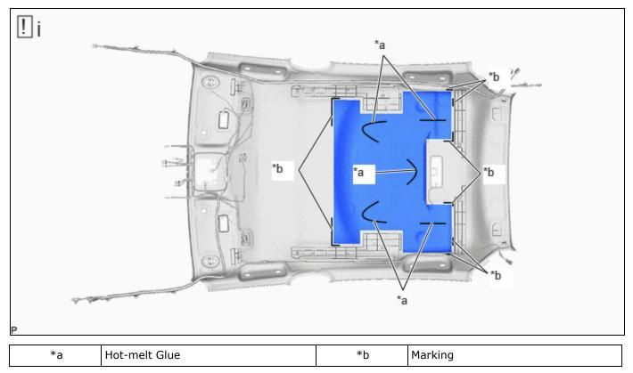
(1) Align the No. 2 roof silencer pad with the markings on the roof headlining assembly and install it using hotmelt glue as shown in the illustration.
