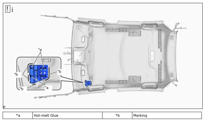
(1) Align the front side rail spacer LH with the markings on the roof headlining assembly and install it using hot-melt glue as shown in the illustration.
