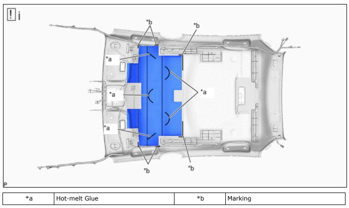
(1) Align the No. 1 roof silencer pad with the markings on the roof headlining assembly and install it using hotmelt glue as shown in the illustration.
