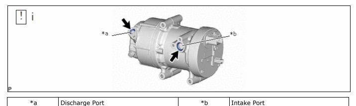
(1) When replacing the compressor with motor assembly with a new one, gradually discharge the inert gas from the service valve, and drain the following amount of oil from the new compressor with motor assembly before installation.
