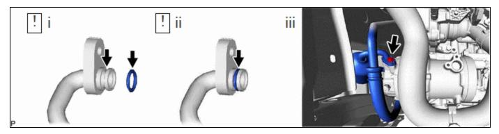
(1) Remove the vinyl tape, and sufficiently apply compressor oil to a new O-ring and the fitting surface of the compressor with motor assembly.
