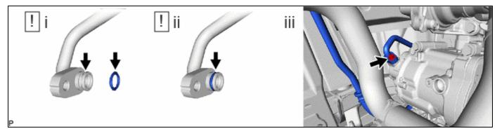
(1) Remove the vinyl tape, and sufficiently apply compressor oil to a new O-ring and the fitting surface of the compressor with motor assembly.
