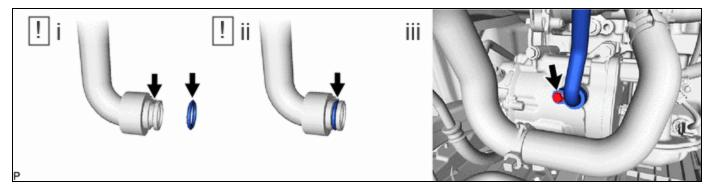
(1) Remove the vinyl tape, sufficiently apply compressor oil to a new O-ring and the fitting surface of the compressor with motor assembly.
