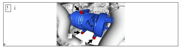
(1) Install the compressor with motor assembly with the 3 bolts.
