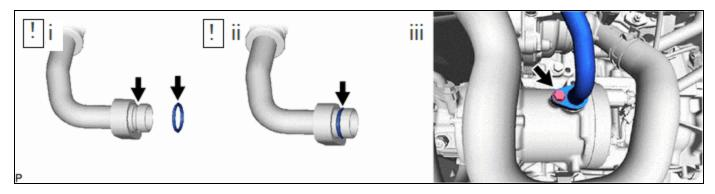
(1) Remove the vinyl tape, sufficiently apply compressor oil to a new O-ring and the fitting surface of the compressor with motor assembly.
