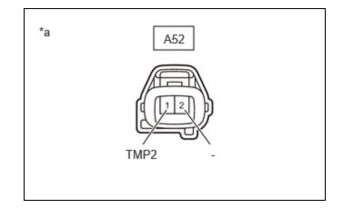
\*a Front view of wire harness connector (to Evaporator Refrigerant Temperature Sensor (No. 2 Air Conditioning Thermistor Assembly))
