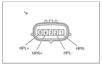
\*a (Cooling Electric Expansion Valve (Cooler Expansion Valve))
