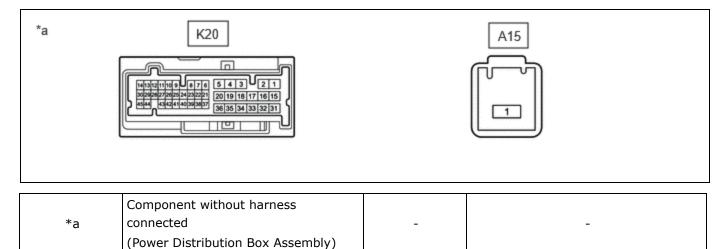
(e) Measure the resistance according to the value(s) in the table below.
