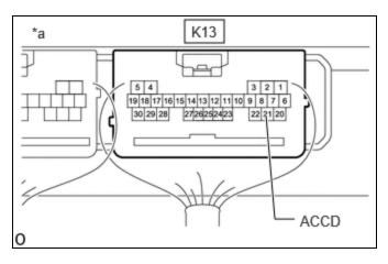
Component with harness connected \*a (Certification ECU (Smart Key ECU Assembly))
