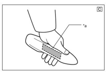
\*a Unlock Sensor (Backside)
