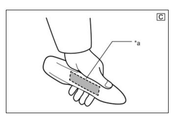
\*a Unlock Sensor (Backside)
