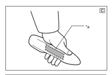
\*a Unlock Sensor (Backside)
