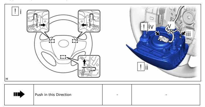
(1) Using a screwdriver with its tip wrapped with protective tape, push in the 3 torsion springs to disengage the 3 pins as shown in the illustration.
