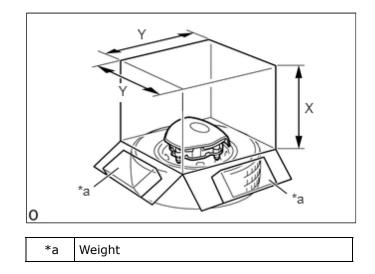
(1) Cover the horn button assembly with a cardboard box.
