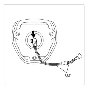
(3) Wind 3 wires around the pins at least 2 times each.
