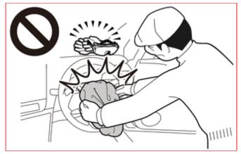
• Do not apply water, etc. to a horn button assembly with a deployed airbag.
