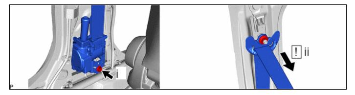
(1) Install the front seat outer belt assembly with the bolt.
