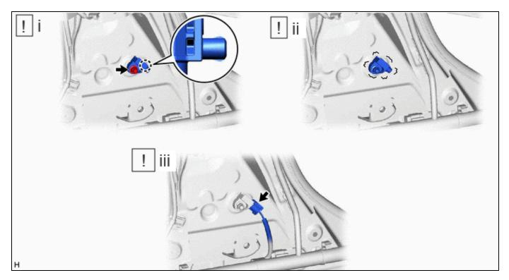
(1) Engage the claw and install the floor side airbag sensor with the nut.
