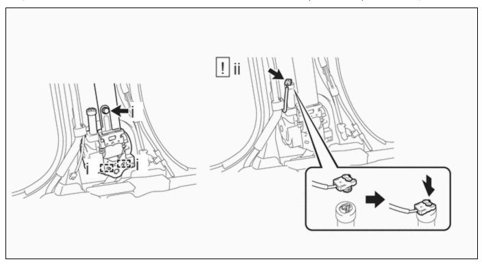
(1) Engage the 2 guides and install the front seat outer belt assembly with the bolt.
