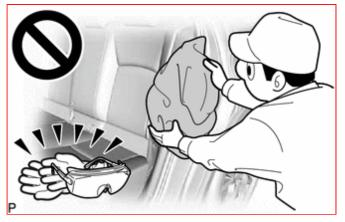
• Do not apply water, etc. to a rear seat airbag assembly with a deployed airbag.
