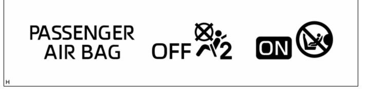
(3) Approximately 6 seconds after the ignition switch is turned to ON, the passenger airbag ON/OFF indicator will indicate ON/OFF depending on the following conditions.
