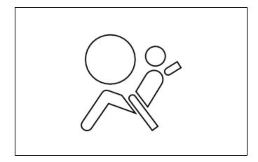
(2) Turn the ignition switch off. Wait for at least 2 seconds, and then turn the ignition switch to ON. The SRS warning light comes on for approximately 6 seconds and diagnosis of the airbag system (including the seat belt pretensioners) is performed.
