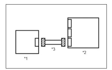
(a) Disconnect the airbag ECU assembly connector.
