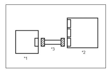
(a) Disconnect the airbag ECU assembly connector.
