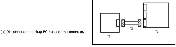
\*1 Front Seat Adjuster Assembly RH (Front Occupant Classification Sensor LH)
