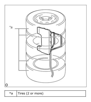
(2) Place at least 2 tires onto the tire to which the lower No. 1 instrument panel airbag assembly is tied. The top tire should have a wheel installed.
